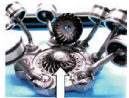
Centre Ball has melted and welded it's self to the fixed gear due to insufficient cooling through loss of refrigerant and/or
